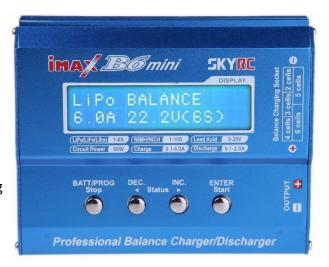
The batteries used in the Seahorse KontikiDrone is a LiPo battery. LiPo Batteries should not be left unattended with charging. Place the LiPo battery on a concrete floor or a metal tray when charging. Some people charge LiPo batteries inside a metal container.
